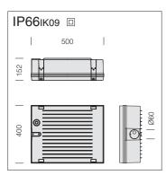
Housing: in die-cast aluminium with latch.
