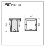
Housing: made of nylon. Frame: in AISI 304 stainless steel. Outer casing: nylon outer casing. Diffuser: tempered glass, 12mm thick, resistant to thermal shock. and mechanical stress up to 2000 Kg.
