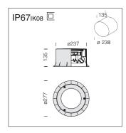
**Housing:** fibreglass aluminium. **Frame:** made of stainless steel AISI 316.
