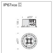
**Housing:** fibreglass nylon with AISI 316.
