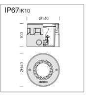
**Housing:** fibreglass nylon with stainless steel AISI 316 frame.
