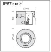
**Housing:** fibreglass nylon with stainless steel AISI 316 frame.
