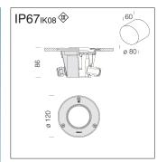
**Housing:** in fibreglass aluminium and stainless steel AISI 316 frame.
