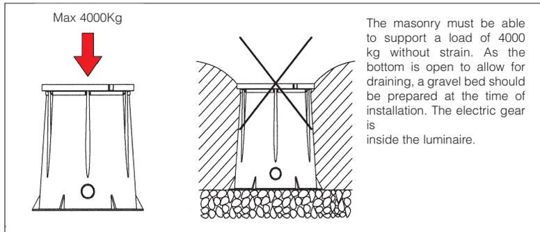
The masonry must be able to support a load of 4000 kg without strain. As the bottom is open to allow for draining, a gravel bed should be prepared at the time of installation. The electric gear is inside the luminaire.
