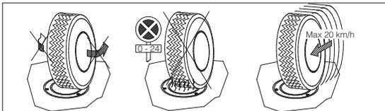
The luminaire can be walked on and can bear vehicle loads.
