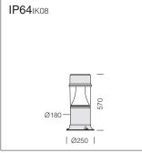
**Housing:** in extruded aluminium, cylindrical section.
