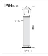
**Housing:** in extruded aluminium, cylindrical section.
