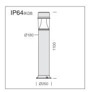
**Housing:** in extruded aluminium, cylindrical section.
