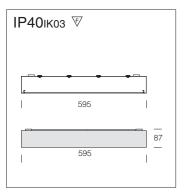
**Housing:** made of sheet steel. **Diffuser:** in frosted plexiglass.
