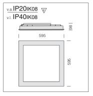
Housing and frame: injection moulded in white polycarbonate, shatterproof and self-extinguishing.
