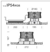
Housing: in extruded 6060 aluminium alloy with 1.5 mm thick steel end caps. Frame in die-cast aluminium for recessed mounting on false ceilings with integrated brackets. Screws and washers in AISI 304 stainless steel.
