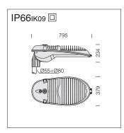
Housing: in die-cast aluminium.
