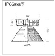
**Housing:** very low magnesium content die-cast aluminium alloy.
