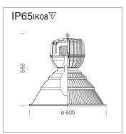
**Housing:** very low magnesium content die-cast aluminium alloy.
